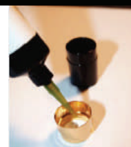
Adhesive applied to aluminium collar
