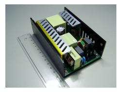
Based upon the experience in design and manufacturing of more than 1 Billion power supplies and battery chargers, FRIWO is offering several interesting features: This OF150 comes with an output voltage of 24 VDC at 6.25 Amp nominal current, other output voltages can be made available.
